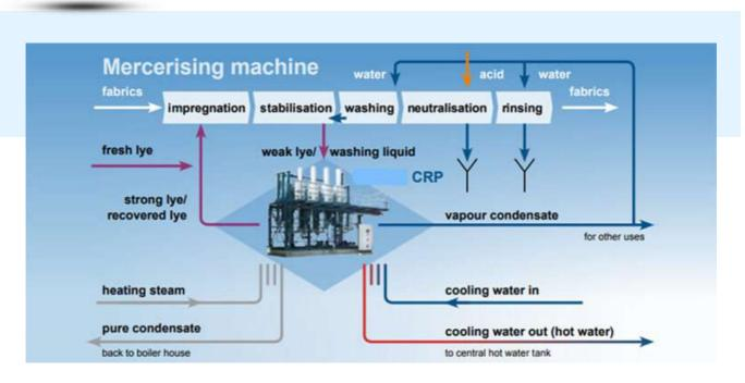
It is a caustic when it goes to the wastewater treatment plant it increases the pH of the wastewater often this makes difficult wastewater treatment process. So, before caustic is sent to the wastewater treatment plant it needs to be neutralised and by recovering the caustic before it
